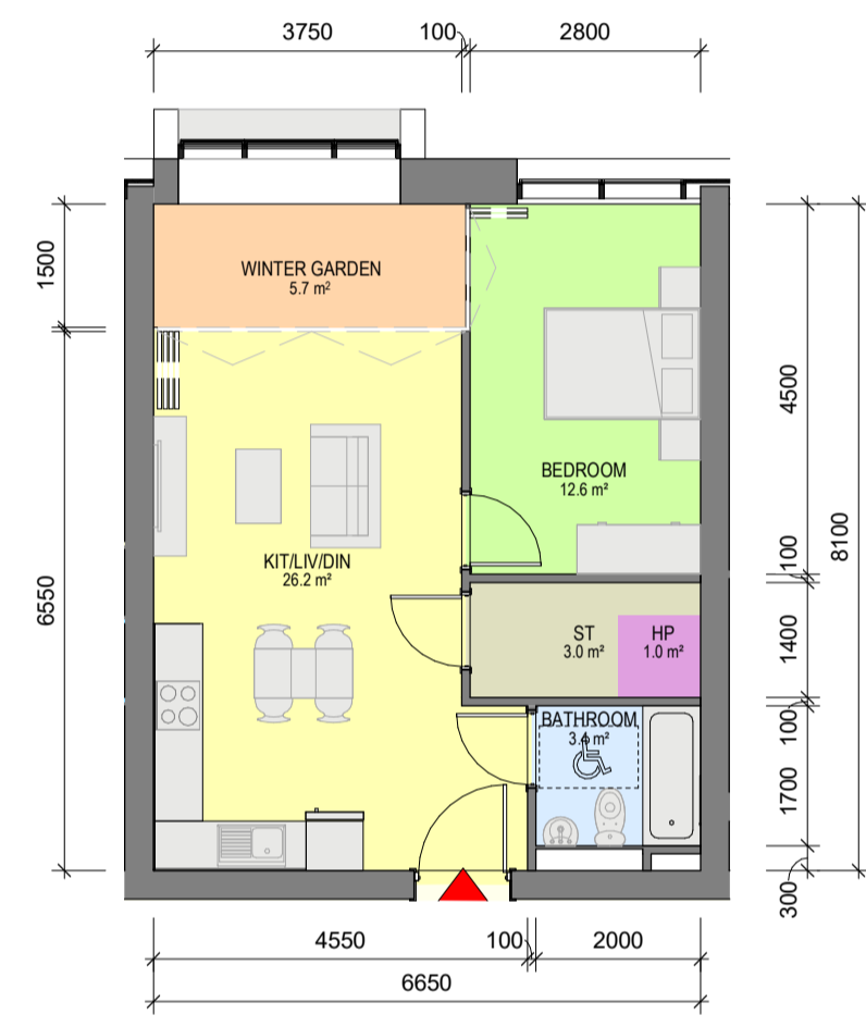
9 Apartment Type 1AM 1 : 100 - 1 BED, 2 PERSON APARTMENT - NET INTERNAL AREA (NIA) Areas shown in plan - GROSS INTERNAL AREA (GIA) : 47.90sqm
