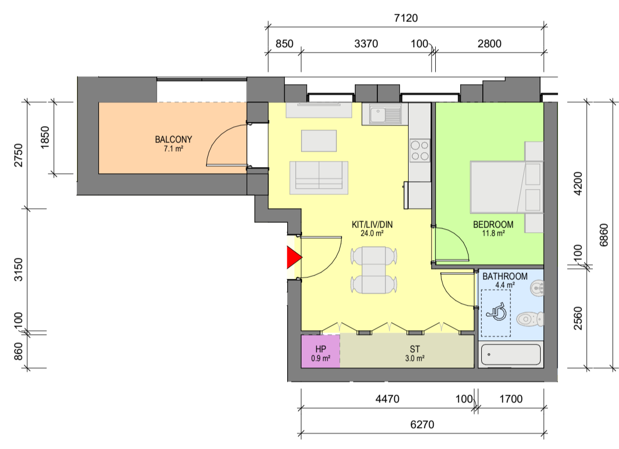
8 Apartment Type 1AL 1 : 100 - 1 BED, 2 PERSON APARTMENT - NET INTERNAL AREA (NIA) Areas shown in plan - GROSS INTERNAL AREA (GIA) : 45.36sqm
