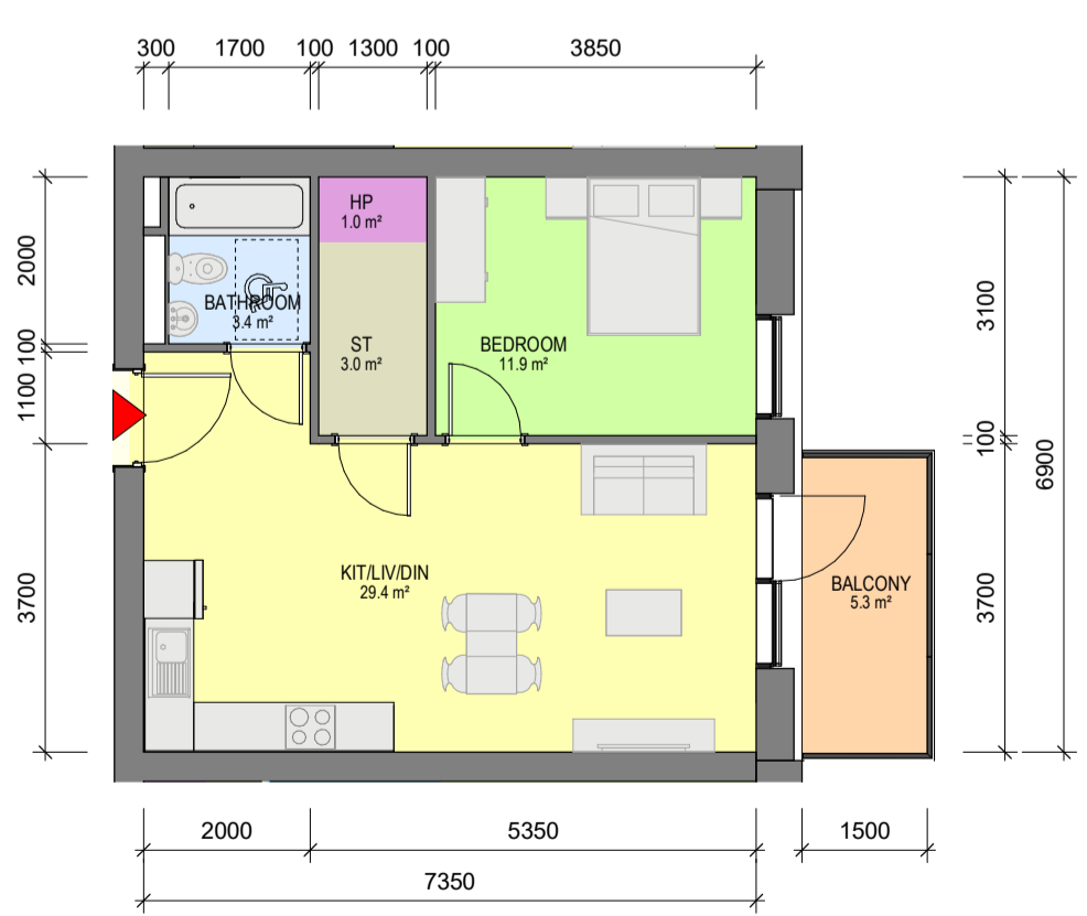
11 Apartment Type 1AO 1 : 100 - 1 BED, 2 PERSON APARTMENT - NET INTERNAL AREA (NIA) Areas shown in plan - GROSS INTERNAL AREA (GIA) : 50.72sqm
