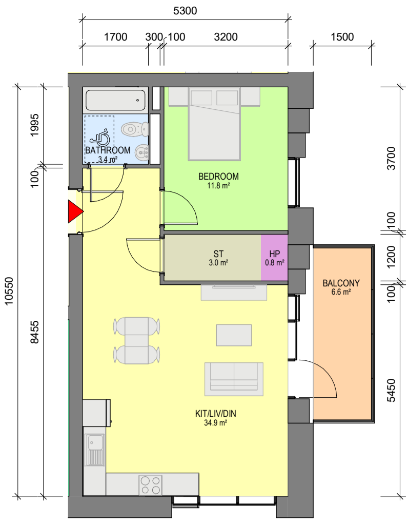
2 Apartment Type 1AF 1 : 100 - 1 BED, 2 PERSON APARTMENT - NET INTERNAL AREA (NIA) Areas shown in plan - GROSS INTERNAL AREA (GIA) : 55.92sqm
