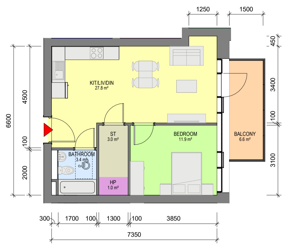
5 Apartment Type 1AI 1 : 100 - 1 BED, 2 PERSON APARTMENT - NET INTERNAL AREA (NIA) Areas shown in plan - GROSS INTERNAL AREA (GIA) : 49.07sqm
